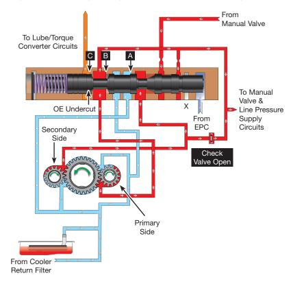
Figure 3 — Tuned Programming: PR Valve Position at Higher Speed/Engine RPM
