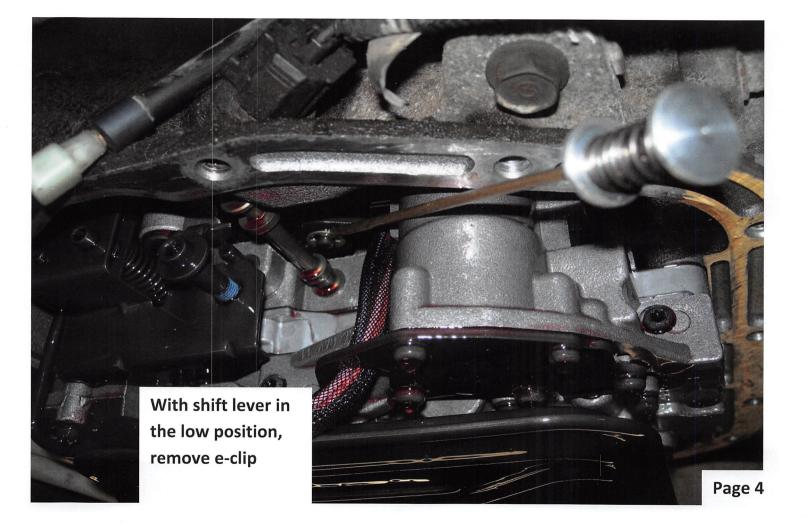
Remove 10 blue painted bolts (yours will not be painted) then lower valve body and remove e-clip
