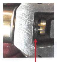
Steel sensor is held into the block with steel clip
