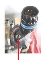
Attach 8-pin connector to 3-4 accumulator housing with T-25 shoulder screw
