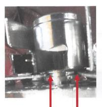
Be sure governor solenoid bracket goes into the outer most groove of the solenoid for proper installation
