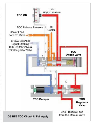
fed to the clutch. Compared to RFE units, this transmission family has a lower max pressure in Drive near 130 psi when in TCC or in 4th Gear. Performance kits will increase that pressure to 150 psi and higher, which is much lower than the RFE family, but can still cause ballooning.
