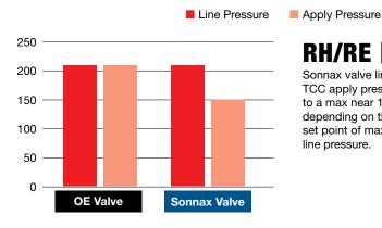
Sonnax valve limits TCC apply pressure to a max near 130 psi depending on the set point of max
