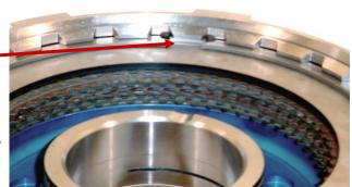
**Step 4** If your clearance is too loose (greater than .050" – 5 plates or, .060" – 6 plates) then add an additional Steel Plate and re-check the clearance.
