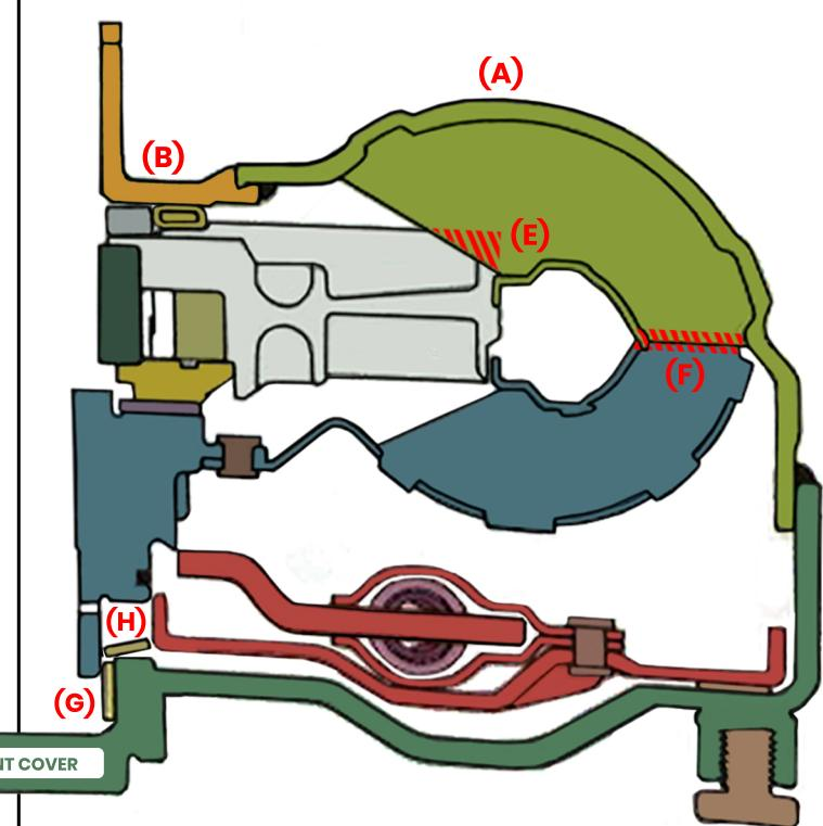
One way to check if a converter is ballooned would be to measure the total height of the assembled converter. Each type of converter should be a specific height. You can see in the above diagram that the converter has a taller height after ballooning.
